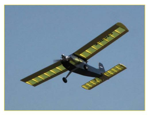
The "Little Rascal" built and flown by Bob Stamm. This is a Sig kit with a 36 inch wingspan circa 1960. Bob has set it up to fly with rudder and elevator using a .061 AP which is similar to the modern day Norvell.
